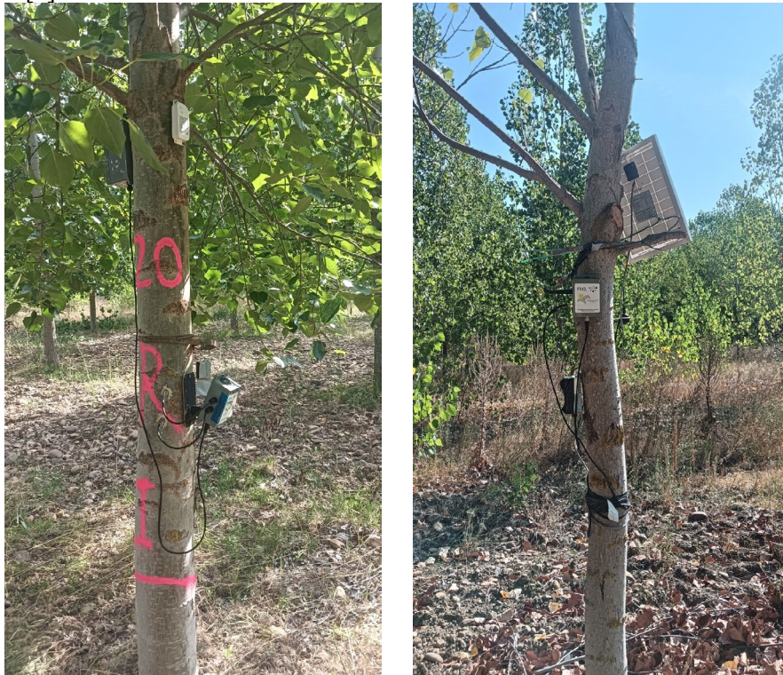
128 Fig. 2. Tree talker TT+ and permanent DBH measuring tape placed on one 129 of the monitored trees (right) and TTcloud (with solar panel and GPRS antenna) 130 display in the study plot. 131
